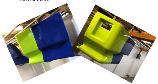
These items were reverse engineered from a supplied sample recreated in an identical resin and the process was complete in 4 weeks from customer order including the supply and installation of the required metalwork.
